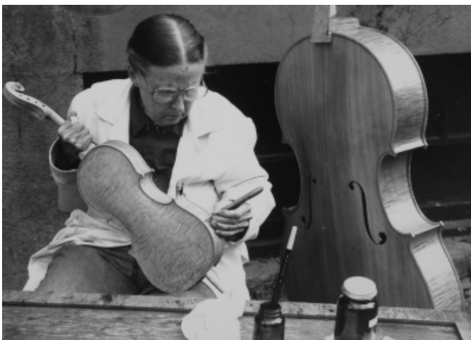
An early photo of Carleen Hutchins varnishing a standard viola. A small bass in the background awaits the brush.
